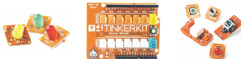
Figure 1: TinkerKit Sensor Shield and modules
